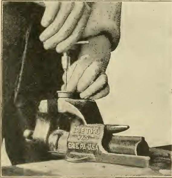
Fig. 76—Using a small tap in a tap wrench
